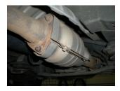
3) At the center of the vehicle, remove the three nuts at the flanged connection behind the catalytic converter. Once the connection is loose, lower the muffler stand and remove the stock exhaust system form the vehicle.
