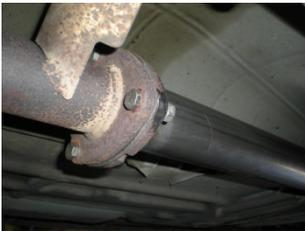
5) Place inlet pipe **#16834S** along with gasket **#GA121** onto the back of the catalytic converter. Using the 3/8" bolts, nuts and washers provided secure the two flanges together and tighten securely. Place a provided 2 1/4" clamp onto the back of this pipe in preparation for the next step.
