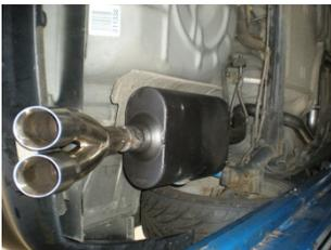
8) Place the **ST448** stainless tip onto the muffler outlet and adjust to the desired position. Tighten the clamp enough to hold, but still allow for adjustment.
