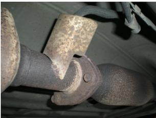
4) At the center of the vehicle, remove the three bolts attaching the factory mid pipe to the rear of the catalytic converter. Once the flange is loose, lower the pipe from the vehicle.
