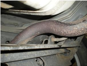
2) In order to remove the stock exhaust system, the system must be cut in half. The best place to do this is just in front of the rear axle.
