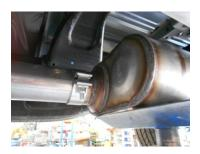
3) Place a supplied 3 ½" clamp over the inlet of the muffler and then slide the inlet of muffler onto the back of the inlet pipe. Use a stand to support the muffler. Tighten the clamp just enough to hold in position.
