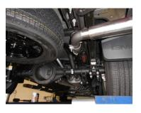
7) Slide the side exit pipes **#86097S** or the rear exit pipes **#86098S** onto the ends of both over axle pipes and place a supplied 2-1/2" clamp onto these slip-fit connections. Tighten just enough to hold in position. Place the two stainless tips **#ST461** onto the exit pipes and tighten them enough to hold position. Rotate the exit pipes and tips to the desired distance from the body or bumper, so that the angle cut on the tips are in the desired location.
