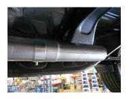
2) If installing the system on a Crew Cab truck with a 6.5' bed, place extension pipe **#36065S** onto the back of the **#36064S** inlet pipe, place a provided clamp onto the slip-fit and tighten enough to hold in position. This extension pipe will not be used on Double Cab or Crew Cab-5.5' bed models.
