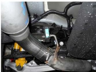
4) Place a provided clamp onto the inlet of muffler **#815430-298** and put up into position on the left side of the vehicle. Slide the inlet of the new Flowmaster muffler up to the tab on the factory pipe. Connect the hanger at the rear of the muffler assembly to the rubber mount on the vehicle and tighten the clamp at the inlet enough to hold, but still allow for adjustment.
