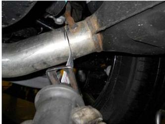
3) To remove the muffler on the passenger side of the vehicle, make a mark on the muffler inlet pipe just forward of the hanger that supports the front of the muffler. Support the muffler with a stand and then using a hacksaw or sawz-all, cut the pipe thru on the mark. Remove the hanger at the front and rear of the muffler from the rubber mounts on the vehicle. Carefully lower the stand and remove the muffler from the vehicle.
