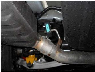
2) At the rear drivers' side of the vehicle, loosen the clamp on the muffler inlet. Support the muffler with a stand and remove the hanger at the rear of the muffler assembly from the rubber mount on the vehicle. Carefully lower the stand and remove the muffler from the vehicle.
