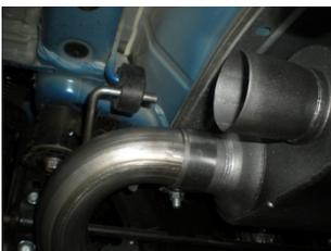
5) Place a provided clamp onto the inlet of muffler **#852583-Z** and place onto the back of mid-pipe **#16815S**. Rotate the muffler so that it is level and support the muffler with a stand. Tighten the clamp on the muffler inlet enough to hold, but still allow for adjustment.
