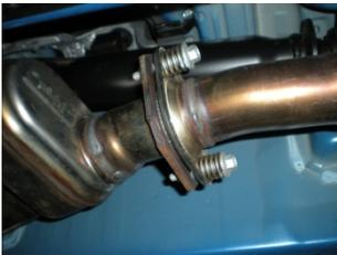
2) Support the rear of the exhaust system with a stand. Remove the two nuts at the flanged connection in the center of the vehicle. Then remove the hanger in the center of the system and the four at the rear of the system from the rubber mounts on the vehicle. With the help of an assistant, carefully lower the stock system from under the vehicle.
