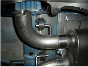
6) Place a provided clamp onto the left muffler outlet. Then put the left exit pipe **#16816S** into position and connect the hanger on the pipe to the rubber mount on the vehicle. After connecting the hanger, slide the pipe into the muffler outlet and tighten the clamp enough to hold, but still allow for adjustment.
