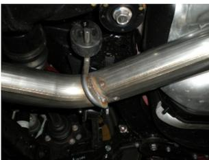
4) Place a provided clamp onto the front of mid-pipe assembly **#16815S** and slide onto the back of the inlet pipe **#16814S**. Rotate the assembly up into its approximate position and connect the hangers on the pipe to their rubber mounts on the vehicle. Tighten the clamp enough to hold, but still allow for adjustment.
