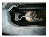
5) Place the clamp of **433HA** over the end of the inlet pipe and connect to the rubber mount on the vehicle. Place the inlet of the muffler thru the clamp and onto the back of the inlet pipe. Support the muffler with a stand and tighten the clamp enough to hold but still allow for adjustment.
