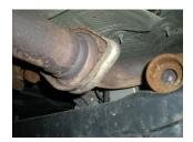
2) Using a 15mm socket, loosen the bolts at the front flange connection behind the catalytic converter.
