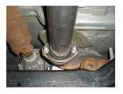
4) Connect the flange on inlet pipe **#26359S** to the flange behind the catalytic converter. Use the supplied 3/8" bolts, nuts and washers and tighten enough to hold but still allow for adjustment.
