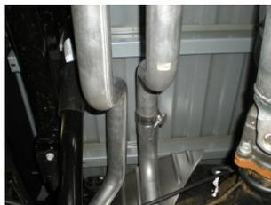
10) Connect the rear section of the left side tailpipe **#16414S** onto the back of the front section by sliding the two sections together at the slip-fit connection over the rear axle. Place the hanger at the rear of the tailpipe into the rubber mount installed in Step 6 above. Tighten the clamp enough to hold, but still allow for adjustment.
