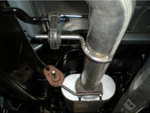
6) Connect the inlet of the muffler **#8530572-Z** to the inlet pipe. Use a stand to support the muffler and install clamp hanger **#392HA** provided in the parts kit onto the inlet of the muffler. Tighten the clamp enough to hold but still allow for adjustment.
