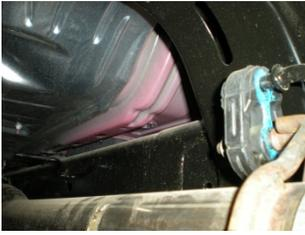
5) On Crew-cab long bed models, there are three hangers between the muffler and the catalytic converter, two with a rubber isolator and one without. Take the rubber isolator from the second hanger from the muffler and place it onto the hanger welded to the frame midway between the converter and the muffler. Slide clamp hanger **#416HA** over the back of inlet pipe **#26332S** and connect to this rubber mount.
