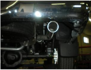
11) Slide either the side exit pipe **#16317S** or the rear exit pipe **#16397S** on the ends of both over-axle pipes. Place a 2 1/2" clamp onto these slip-fit connections. Tighten enough to hold, but still allow for adjustment. Place the two stainless tips **#ST396** onto the exit pipes and tighten the clamps enough to hold, but still allow for adjustment. Rotate the exit pipe and tip to the desired distance from the fender or bumper and so angle cut on tips are in the desired location.
