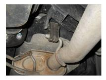
3) Support the rear muffler with a stand, then separate the four hanger rods from their rubber mounts on the vehicle. Carefully lower and remove the system from under the vehicle.
