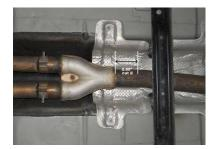
2) Measure and cut the single factory pipe at a point 2" behind the weld at the back of the factory Y-pipe. Use a die grinder or file to de-burr after cutting.
