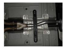
4) Begin by placing a clamp onto the new inlet pipe **#16625S**. Now place the inlet pipe onto the back of the factory Y-pipe. The rear of the inlet pipe should be positioned so that it is offset to the drivers' side.
