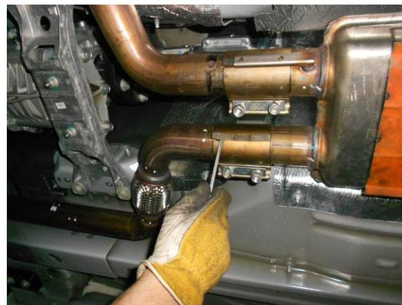
3) Support the center resonator with a stand and loosen the four nuts at the two band clamp connections at the resonator inlet. Using a screwdriver, pry up the clips on the clamp body to release the clip from the tab on the inlet pipes. Slide the clamp assemblies slightly back to clear the tabs. You can now lower the rear of the resonator and slide the assembly to the rear of the vehicle to remove. Lower the resonator from the vehicle and set aside.
