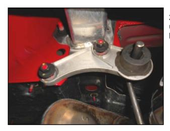
2) Support the rear of the system with a stand and using a 15mm socket or wrench, remove the two hangers at the rear of the system.
