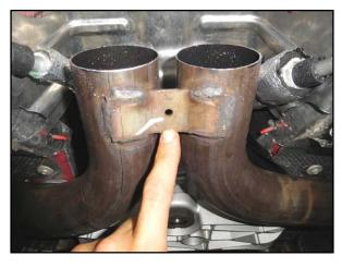
5) Carefully deburr the ends of the front pipes where cut with a file or die grinder. The next step will be to remove the brace between the two front pipes.
