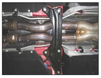
3) Using a 13mm socket or wrench, remove the five bolts securing the body brace to the bottom of the vehicle.
