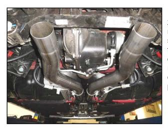
2) Place a provided 3.00" clamp onto the slip-fit of mid pipe #26614S and slide onto the back of the left side Scavenger outlet. Connect the hanger on the pipe to the rubber mount on the vehicle and tighten the clamp enough to hold in place. Repeat this step on the right side of the vehicle with mid pipe #26615S. You can now follow the installation section of the instructions provided with your new Flowmaster axle-back system.
