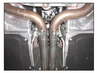
1) Place a supplied 2 ¾" clamp onto the inlets of Scavenger assembly **26611S**, place the assembly onto the front inlet pipes and slide on approximately 3.00". Be sure the Flowmaster embossing in the center of the assembly is facing the ground. Re-install the body brace and tighten securely.
