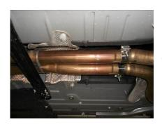
2) Begin by placing a supplied 2 ½" clamp onto each of the slip fits on Scavenger pipe #86337M. Place the Scavenger pipe onto the back of the stock head pipes (make sure the Flowmaster embossing is facing the ground). Level and center the assembly in the drive line tunnel and support with a stand. Tighten the two clamps enough to hold, but still allow for adjustment. Reinstall the two body braces onto the vehicle and tighten securely.
