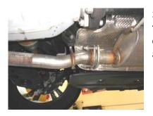
3) Using a 13mm socket, unbolt the left tailpipe assembly at the flanged connection at the rear of the muffler. Slide the three hanger rods out of the rubber mounts on the vehicle and remove the left tailpipe assembly.
