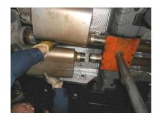
3) Place a supplied 2 ½" clamp onto the inlet of each #742541-Z muffler. Then fully slide the mufflers onto the back of the Scavenger pipe assembly and support with stands. Level the mufflers and tighten the clamps enough to hold, but still allow for adjustment. **Note:** The protective plastic wrap has been left on the mufflers to protect their finish, please remove prior to starting the vehicle.
