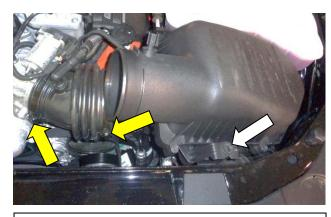
4. Loosen the hose clamps → which secure the factory intake tube to the throttle body and air-box. Detach from the air-box by compressing the intaketube bellows towards the engine. Remove the bolt → for the factory air-box on the front cross frame.
