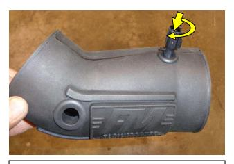
11. Assemble the FM intake tube as shown using the two provided rubber grommets. Install the stock air-temperature sensor into the small grommet as shown by pressing in and twisting clockwise.
