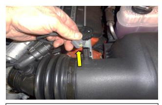
2. Carefully disconnect the air temperature sensor connector by depressing the rocking tab on the back of the plug and pulling straight off.
