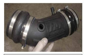
12. Loosely assemble the provided silicone-rubber couplers and corresponding hose clamps onto the FM intake tube as shown.
