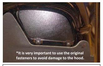
17. Using the original fasteners\*, install the vent cover over the screen as shown and tighten securely. Reattach the negative ground clamp to the battery, recheck all connections, fasteners and fitment. Enjoy!
