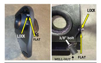
9. Loosely attach the two provided metal brackets to the heat shield using the ¼" cap screws/nuts and corresponding flat and lock washers ⇒ and the well-nut with corresponding 3/8" bolt ⇒as shown.
