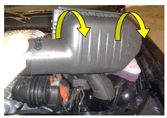
5. Remove the factory air-box assembly by lifting up and rolling forward simultaneously. Then, remove the factory intake tube from the throttle body. NOTE: We highly recommend that customers retain their factory air intake system.
