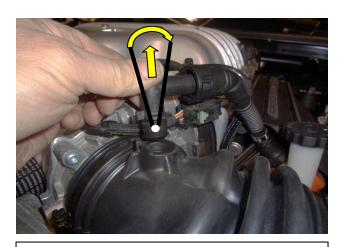
3. Disconnect the crank-case vent hose fitting from the stock intake tube by gently pulling straight up in an orbital motion. To make removal easier, spray a lubricant into the rubber connection point to act as a release agent for the fitting barbs.
