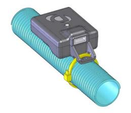
7. Connect the female connector on the Delta Boost module to the factory male sensor.
