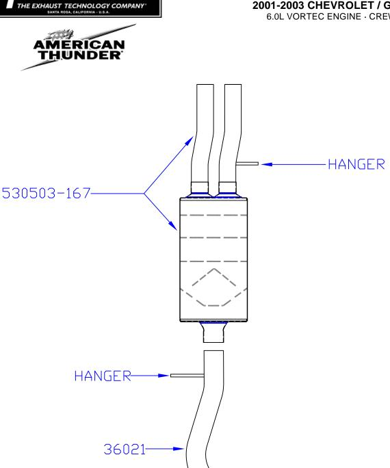
**HANGER** PACKING LIST QTY. PART# DESCRIPTION 530503-167 MUFFLER 1 36021 **OVERAXLE PIPE** 1 PK393 PART KIT HANGER KEEPER 3.50" CLAMP 3 MC350SB
