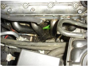
**Step 10.** Install your new header assemblies, plug in the O2 sensors before install, with the supplied gaskets and attach using the supplied header bolts with a 10mm socket to the manufacturers torque specifications.
