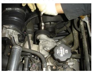
**Step 6.** Release the pressure on the drive belt tensioner with a 15mm socket and remove the serpentine belt.
