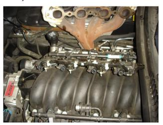
**Step 9.** Using a 13mm socket unbolt both manifolds and remove. While removing both manifolds disconnect the O2 sensor plug. Unbolt and remove the O2 sensor cable from the OEM manifold using a 7/8" wrench and bolt it onto your new header assemblies.
