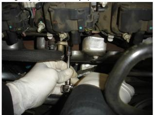
**Step 3.** Unbolt and remove the A.I.R. pipe on the passenger side using a 10mm socket.
