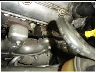
**Step 4.** Using a 15mm socket remove the dipstick assembly.
