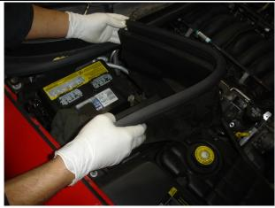
**Step 1.** Before removing the OEM manifold system, first disconnect the battery using a 10mm socket. Then remove the rubber battery enclosure to gain more access to the OEM manifold. Remove the engine covers by gently pulling to disengage it from the rubber grommets.
