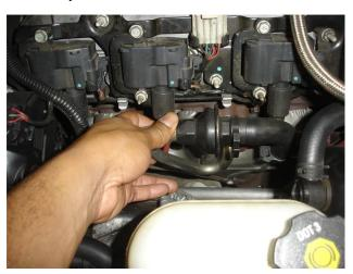
**Step 5.** Disconnect the hose from the A.I.R. pipe on the driver side and remove.
