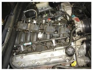
**Step 2.** Remove all spark plug wires from the coils and the plugs, and then set aside. On the passenger side unbolt the coil pack bracket using a 10mm socket and gently flip the assembly up towards the motor.
