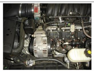
**Step 7.** Using a 15mm socket unbolt the alternator and remove. After alternator has been removed repeat passenger side process to remove the coil pack bracket.
