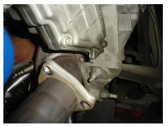
**Step 8.** Using a 15mm socket unbolt both catalytic converters from the OEM manifolds.
