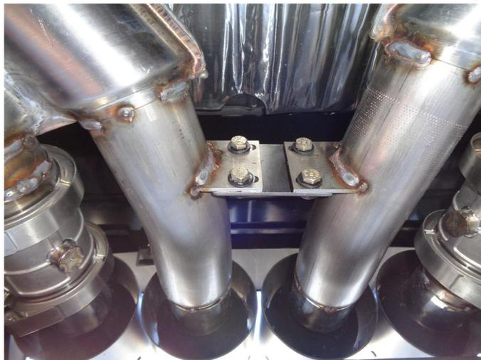
**Step 8.** Locate both OEM hanger brackets to each Tail Pipe Assembly. Next, loosely attach both assemblies to the Inlet Pipe Assembly outlets using the supplied 3.00" clamps. Using the supplied nuts, bolts and washers connect the two hanger brackets that will link both sides together. Reconnect each wiring harness connector to the valve motors. Reinstall the rear valence in the reverse order of the removal process.
