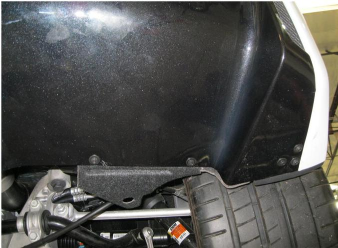
**Step 2.** Then you will need to remove the five 7mm bolts on both sides of the valence underside. Remove two 10mm bolts above the exhaust tips. The valence is fastened from the backside with molded-in plastic tabs. Release the six tabs from the valence by gently pulling each tab from the valence.
