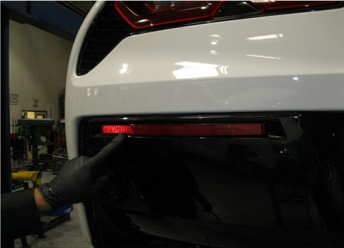
**Step 1.** To remove the OEM exhaust system you will first need to remove the rear valence. To do so you will need to remove The two 10mm bolts behind each reflector, the two 10mm bolts behind the license plate and two more 10mm bolts just underneath the license plate.
