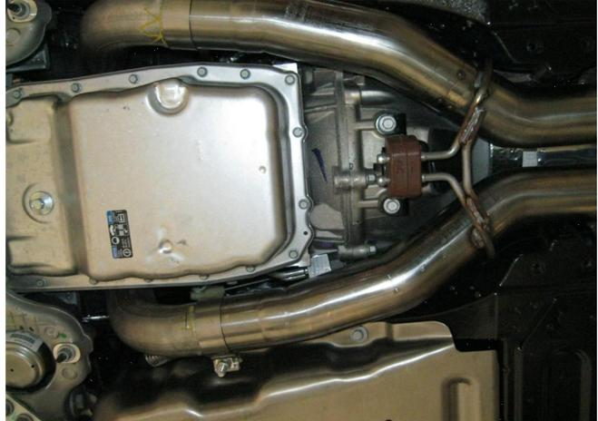
**Step 4.** On vehicles with automatic transmission you will need to disconnect the shift linkage located on the drivers side of the transmission.
