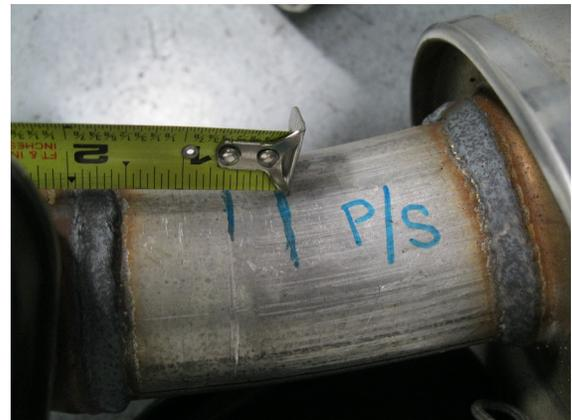
Step 3: Begin removing the OEM exhaust system by cutting both pipes going into the muffler assemblies. Measure and cut 2.0" driver side, 1.75" Passenger side, behind the exhaust valve welds as shown. Next extract the hangers from the rubber insulators and remove the OEM mufflers. Retain rubber insulators and as they will be used to install the new system
