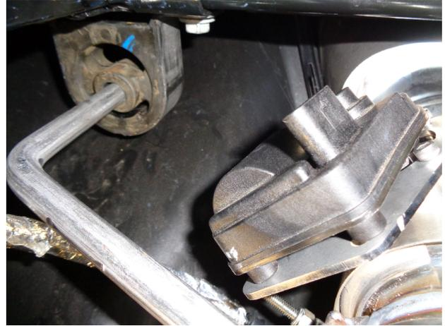
Step 6: If your vehicle has valves re-connect the wiring harness plugs to the Valve motors, re-install the rear valance.
