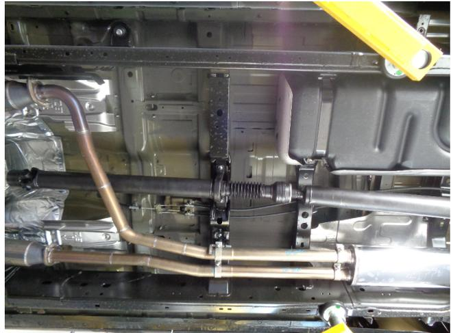
Step 3: Next loosely fasten both Extension Pipes to the Inlet Pipe Assemblies using the supplied clamps.
