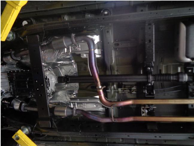
Step 1: To remove the OEM system first unbolt both inlet pipes at the catalytic converter flange junctions. Working front to rear disengage all welded hangers from the rubber insulators. The OEM exhaust system can now be removed in one piece. Be sure to retain all mounting hardware as it will be needed to install your new MAGNAFLOW system
