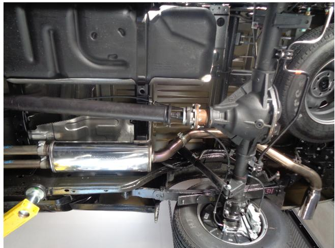
Step 4: Loosely attach the Muffler Assembly to the two Extension Pipes using the supplied clamp and engaging the welded hanger to the rubber insulator. Install the Tail Pipe Assembly the same way.
