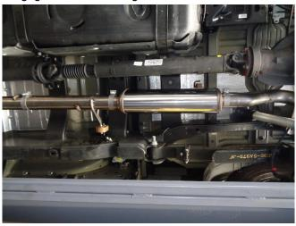
Step 5: If required add the 19.25" Extension Pipe. Loosely attach the Extension Pipe Assembly using the supplied clamp[s]. Engage the welded hanger to the rubber insulator.
