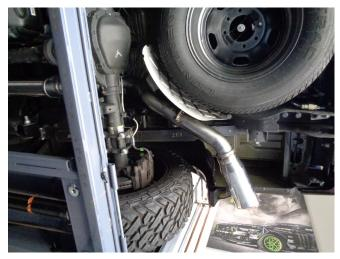
Step 6: Finish by loosely installing the Tail Pipe Assembly using the supplied clamp. Install the welded hanger to the rubber insulator.
