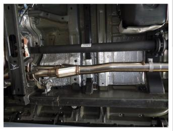
Step 4: Begin installing your new system by loosely attaching the Inlet Pipe Assembly to the catalytic converter outlet pipes using the OEM hardware. Engage the welded hanger to the rubber insulator.
