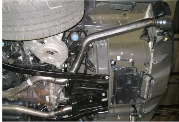
**Step 3.** Next attach both Tailpipe Assemblies to the Inlet Pipe Assemblies using the supplied 2.50" clamps and fitting the hangers into the rubber insulators.
