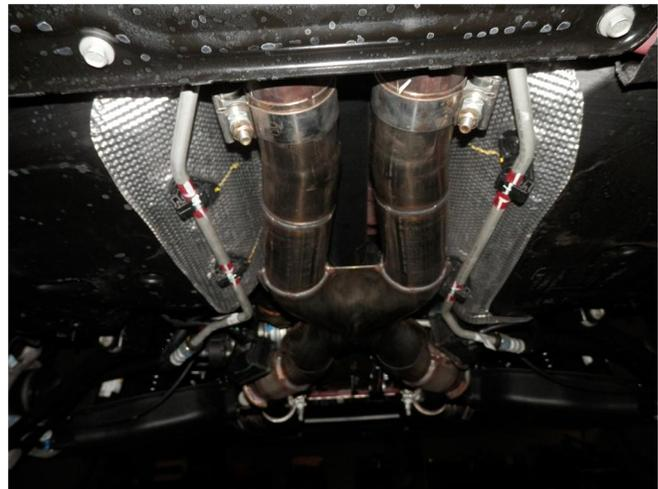
**Step 4.** Begin installation of the new system by sliding the X-Pipe Assembly inlets onto the cut outlets of the OEM exhaust and loosely fasten with the supplied 2.75" clamps. (at this time slide the loose end of the cut heatshield under the clamps before tightening). Fit hangers into rubber insulators.
