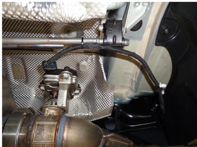
**Step 6.** To re-attach the plug to the valve motor you will need to release the loom from its mounting point on the inner body wall. Attach the connector to the valve then use one or both of the supplied Zip Ties to secure the loom to the hanger as shown,.
