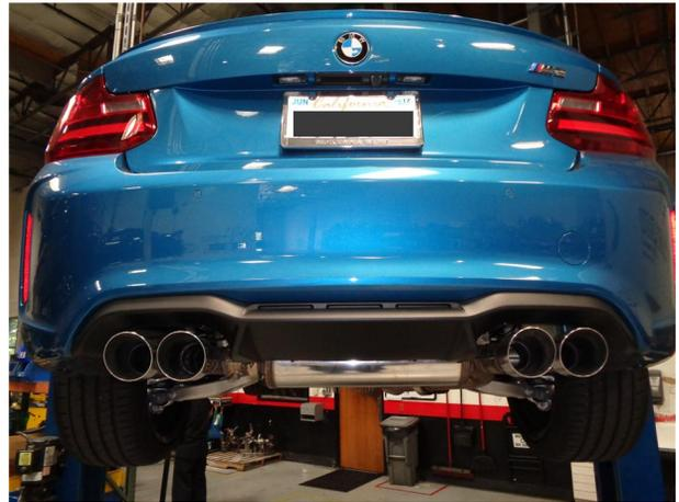
**Step 7.** Once a final position has been chosen for the new system, evenly tighten all clamps from front to rear using the torque specifications on page one of the instructions. Inspect all fasteners after 25-50 miles of operation and re-tighten if necessary.
