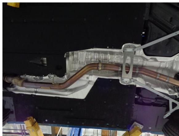
**Step 4.** Next fasten the Resonator Assembly to the inlet pipe using the supplied 3.00" clamp.
