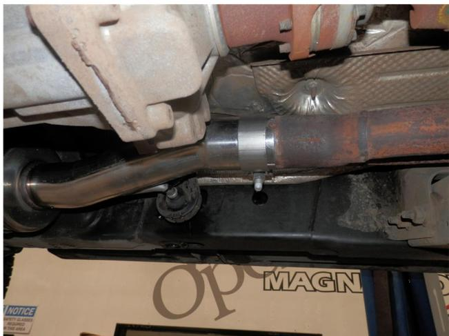
**Step 3.** Begin installation of your new MAGNAFLOW system by attaching the Resonator Assembly to the catalytic converter outlet using the OEM band clamp. Align the locating peg with the notch in the inlet pipe. Engage the welded hanger to the rubber insulators. Keep all fasteners and clamps loose until final adjustment.
