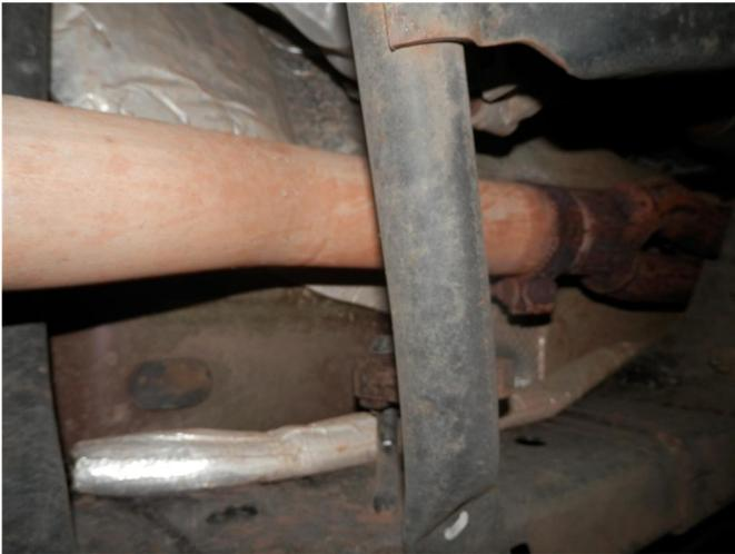
**Step 1.** Begin removal of the OEM exhaust system by loosening the band clamp attaching the exhaust to the catalytic converter. Do not discard or damage the OEM fasteners or rubber insulators as they will be used to install the new system.
