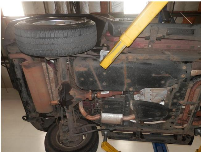
**Step 2.** Disengage hangers from rubber insulators and remove the OEM exhaust.
