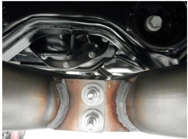
**Step 3.** Next attach the Mid-Pipe Assemblies to the Resonator Assembly using the supplied 2.50" clamps. At this time also use the supplied 5/16" fasteners to connect the Mid Pipe Assemblies.
