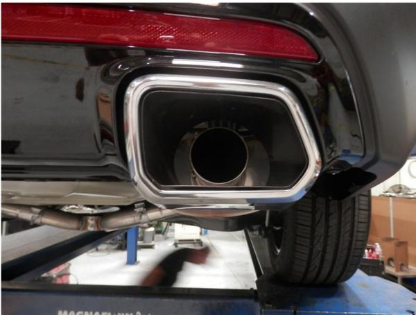
**Step 4.** Complete the installation by attaching the Muffler Assemblies to the Mid-Pipes using a 2.50" clamps and fitting the tailpipes into the openings in the rear valance and the hangers into the rubber insulators.
