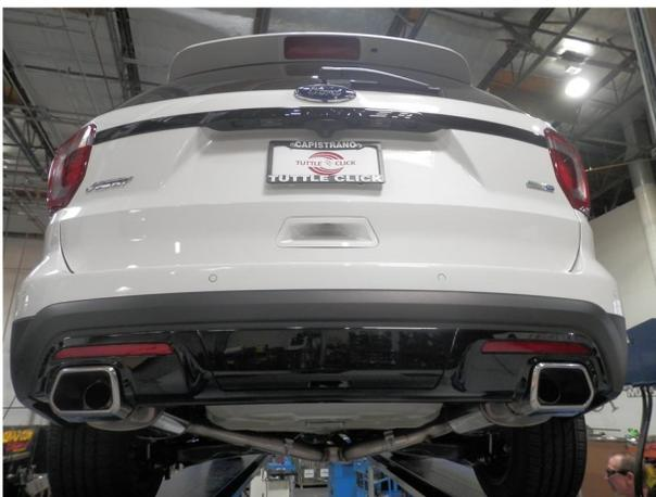
**Step 5.** Once a final position has been chosen for the new exhaust system, evenly tighten all clamps from front to rear using the torque specifications on page one of the instructions. Inspect all fasteners after 25-50 miles of operation and re-tighten if necessary.
