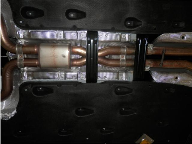
**Step 1.** Begin removal of the OEM exhaust system by detaching the two black cross braces from the underside of the vehicle and both tube braces from the resonator assembly.
