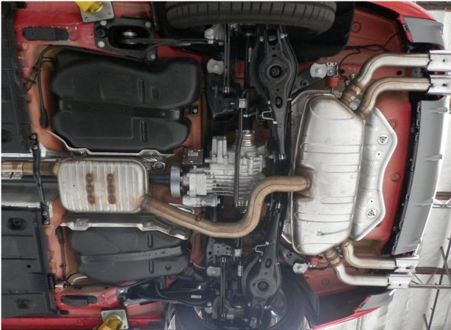
**Step 2.** To remove the OEM exhaust system you will need to loosen the clamp at the vehicles inlet pipe. Working from front to rear disengage all welded hangers from the rubber insulators. Retain all mounting hardware as it will be needed to mount your new MAGNAFLOW system.
