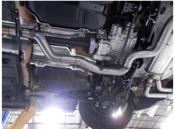
**Step 5.** Loosely Install the Inlet Pipe Assembly to the OEM slip clamp. Engage the welded hangers to the rubber insulators.
