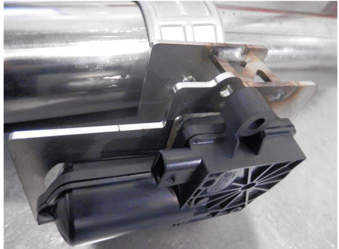
**Step 4.** Before installing your new exhasut system attach the OEM valve motors to each valve using the supplied hardware. The alignment spring on the motor will need to be engaged into the keyway slot of the new valves.
