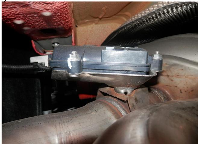
**Step 3.** Once the OEM system has been removed undo three nuts attaching each exhaust valve motor to the valve and remove.
