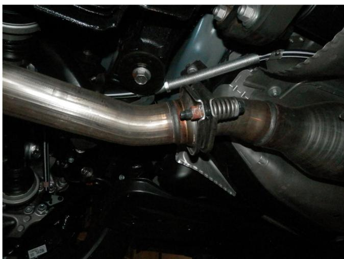
**Step 1.** To remove the OEM exhaust system you will first need to remove the four spring loaded bolts at the flange junction that attach the OEM muffler assemblies to the vehicles catalytic converters. Disengage all welded hangers from the rubber insulators. Be careful not to damage any mounting hardware as it will be needed to mount your new system.
