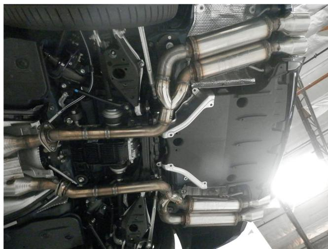
**Step 2.** Begin installation of the new system by fastening the inlet flanges of each Muffler Assembly to the outlet flanges of the catalytic converters using the OEM spring and bolt along with the supplied hardware. Locate the each welded hanger into the OEM rubber insulator.
