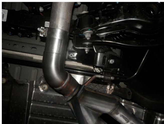
**Step 4.** Loosely install both Tailpipe Assemblies using the supplied clamps. Locate all welded hangers to the OEM rubber insulators.
