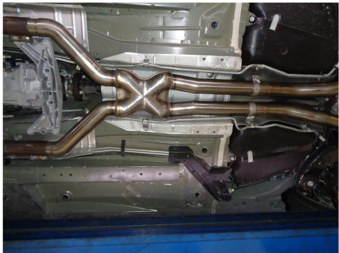
**Step 2.** Begin installing the new system by loosely attaching the inlets of the X-Pipe Assembly to the catalytic converter outlets using the OEM clamps.
