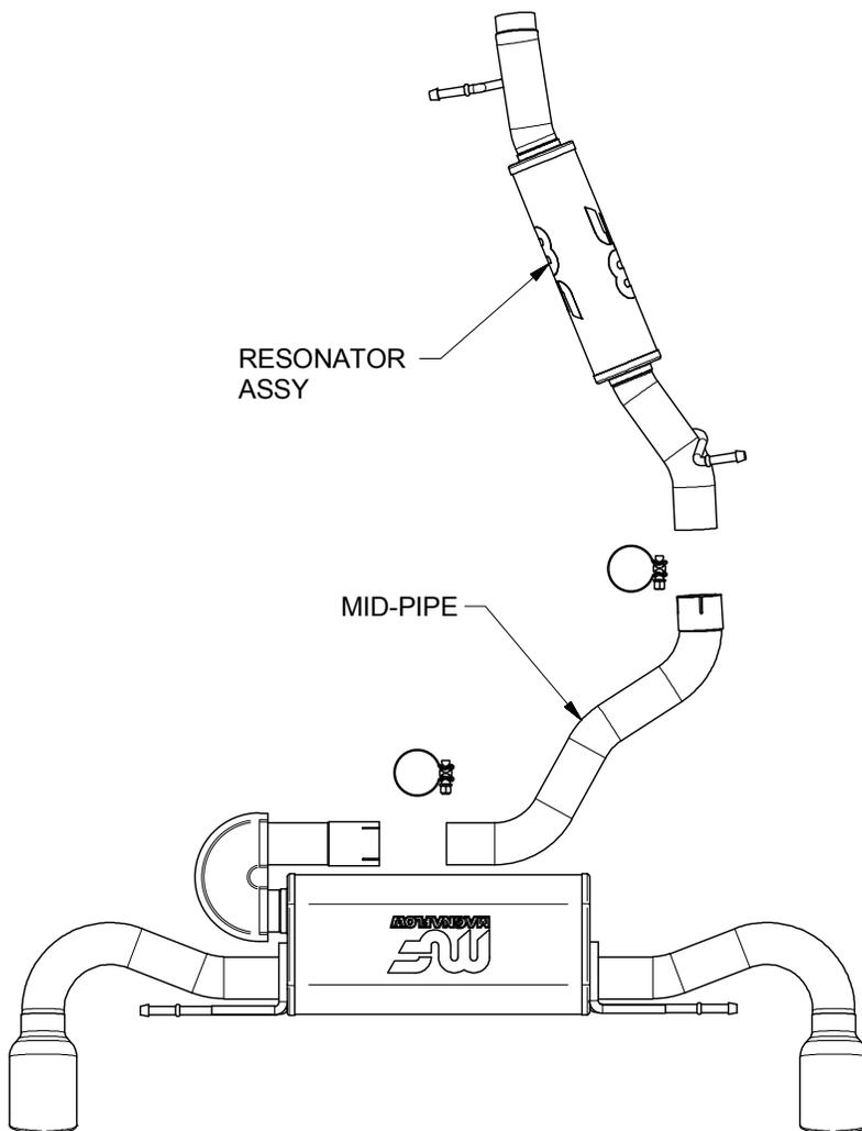
**Step 1:** (Carefully read all instructions before installation) Begin removal of the OEM exhaust system by loosening the OEM clamp located behind the catalytic converter. Do not damage or discard the OEM clamp nor rubber insulators, as they will be reused to mount the new system. Disengage the welded hangers from the OEM rubber insulators and remove the entire OEM exhaust system.
