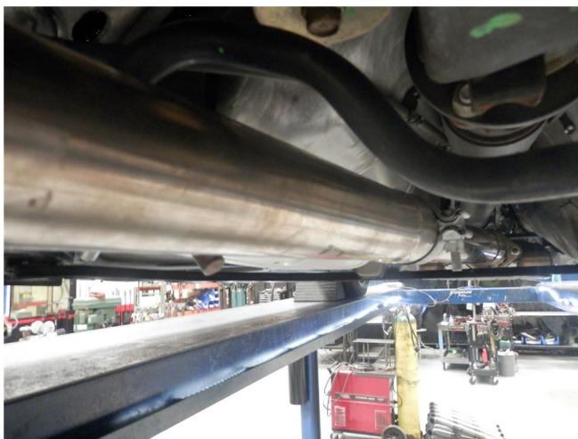
**Step 3.** Begin installation of your new MAGNAFLOW system by attaching the flanges of the Inlet Pipe Assembly to the catalytic converter outlet using the OEM hardware. Keep all fasteners and clamps loose until final adjustment.
