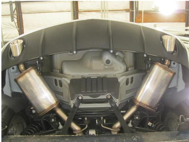
**Step 5.** Finish by attaching the Muffler Assemblies to the extension pipes using the supplied 2.50" clamps and fitting the hangers into the rubber insulators. Replace crossmembers and chassis stiffeners.
