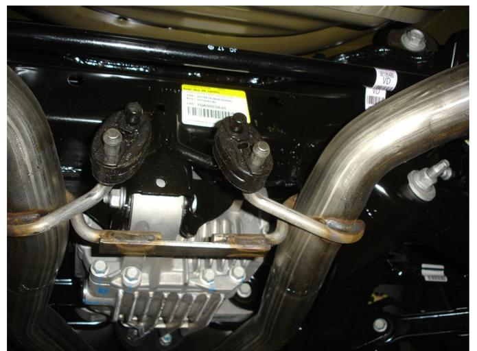
**Step 1.** Begin by removing the two front crossmembers and the two rear chasis stiffeners by the muffler inlets. This will allow access to the exhaust system.
