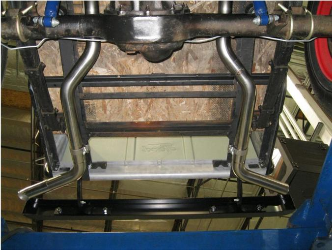
**Step 5.** Once fitted, the Tail Pipes may need to be cut to the desired length. The supplied polished tips may then be welded into position.
