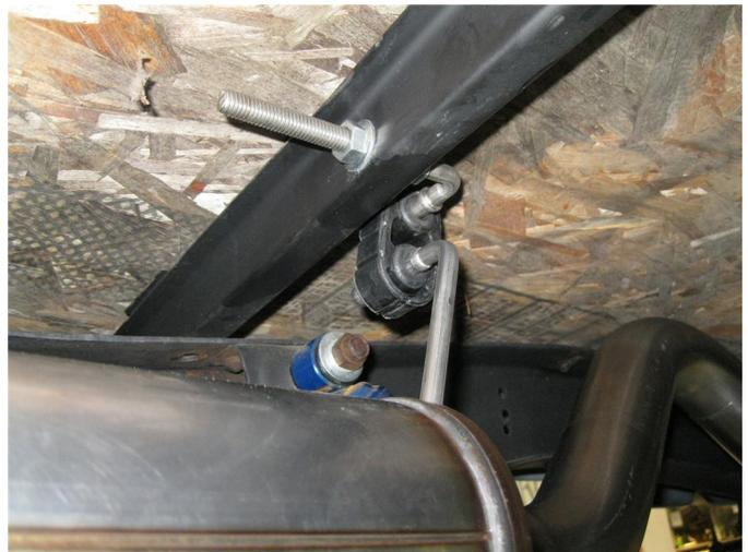
**Step 3.** With the new system loosely installed you will see where the welded hangers on the Muffler Assemblies locate to the vehicles chassis. You will need to drill a hole in the chassis to locate the supplied threaded hangers and secure with the nuts in the hardware kit as shown. Next attach both hangers using the supplied Rubber Insulators.
