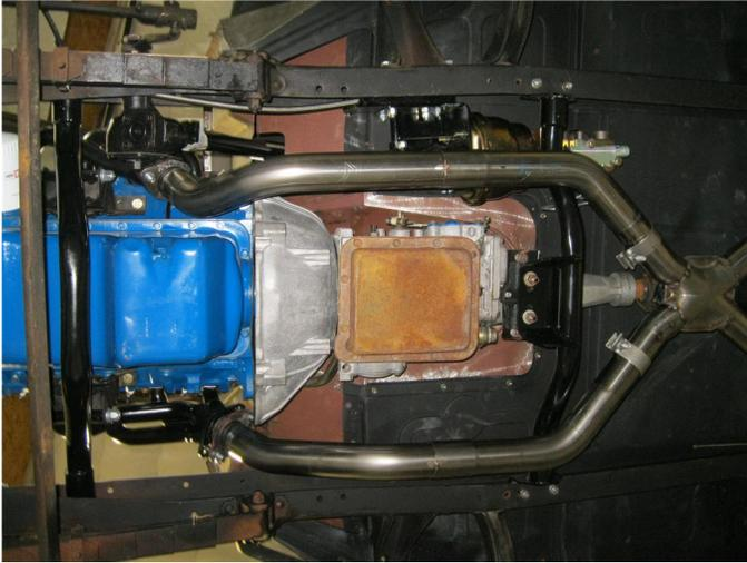
**Step 1.** Begin by removing the existing exhaust system. Depending on the down pipes you have from the headers you will need to cut both the new Inlet Pipes to fit. Slip the Inlet Pipes outlets into the X-Pipe Assembly's inlet pipes. Loosely secure using the supplied clamps.
