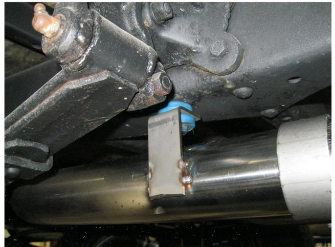
**Step 4.** The welded bracket on each Over Axle Pipe needs to be attached to the chassis also. A hole will have to be drilled to locate the supplied mounting hardware and rubber grommet as shown.
