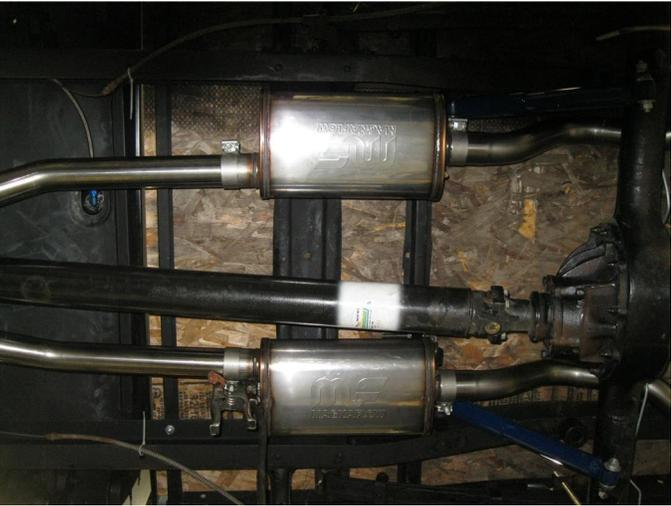
**Step 2.** Loosely install both Muffler Assemblies, Over Axle Pipes and Tail Pipes in a similar fashion using the supplied clamps.
