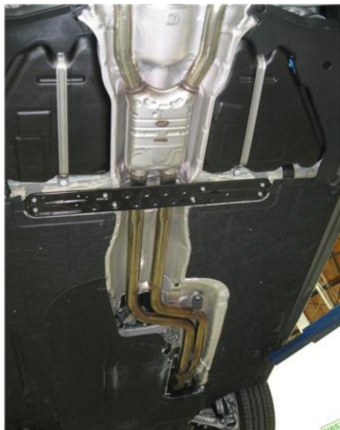
**Step 1.** To allow for extraction of the OEM system you must first remove the underside cross brace. Next loosen the clamp at the outlet of the catalytic converter. Working front to rear detach all hangers from rubber insulators and remove the system. Retain rubber insulators and clamp as they will be re-used the mount the new system.
