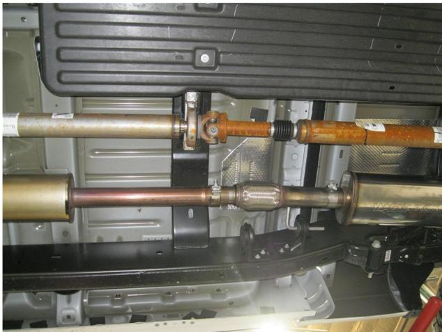
**Step 2.** To begin, fasten the Inlet Pipe Assembly to the catalytic converter using the OEM clamp assembly and by fitting the welded hanger into the OEM rubber insulator (Leave all clamps and fasteners loose for final adjustment of the complete system.) Install the Muffler to the Inlet Pipe Assembly using the supplied 3.00" clamp and fitting the hanger. Next install the Tailpipe Extension Assembly to the Muffler in the similar fashion using the supplied 2.50" clamps.
