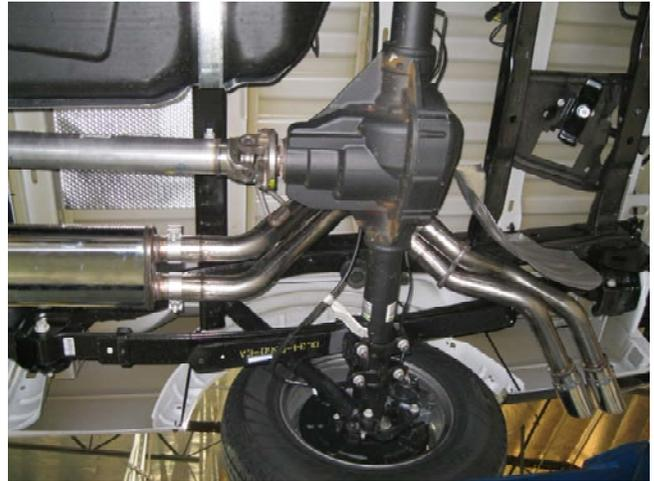
**Step 3.** Finish by installing the Tail Pipe Assembly to the Tail Pipe Extension Assembly using the supplied 2.50" clamps, fitting the welded hanger into rubber insulator.
