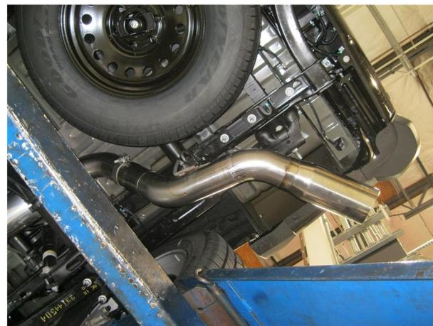
**Step 4.** Finish by installing the Tail Pipe Assembly to the over axle Resonator assembly using the supplied 4.00" clamp, fitting the welded hanger into rubber insulator.
