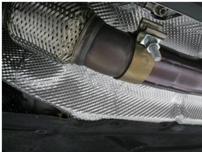
**Step 3.** Begin installing your new system by first attaching the OEM hanger assemblies you removed to the new system. At this stage you may also replace the underbody cross-member. Next, loosely secure the Inlet Pipe Assembly to the OEM flex pipe outlet using the supplied clamp.
