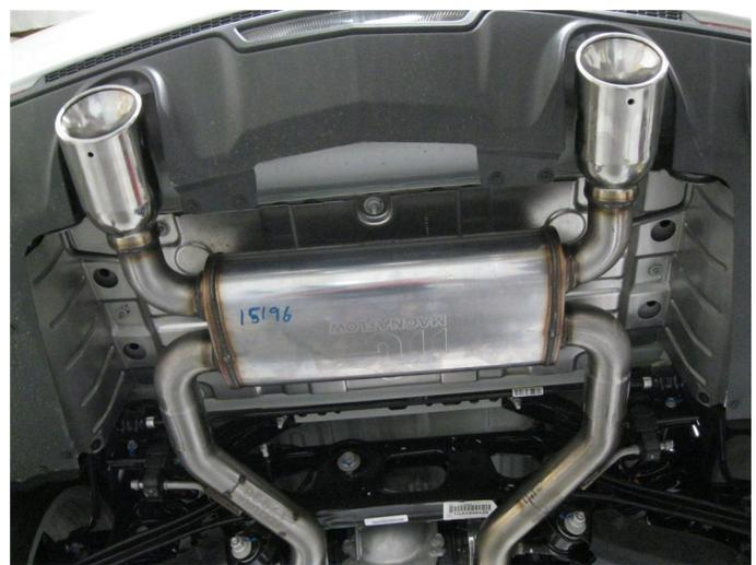
**Step 3.** Next Install the Muffler Tail Pipe Assembly to the outlets of the Inlet Pipe Assemblies using the supplied 2.50" clamps. Insert hangers into rubber insulators.
