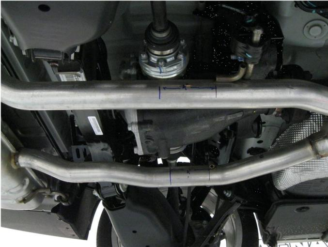
**Step 1.** To remove the OEM exhaust system you will first need to cut both pipes between the front and tail pipe mufflers 4.00" behind the welded hangers as indicated. Disengage all welded hangers from the rubber insulators and remove the OEM system. Do not damage or discard the rubber insulators or fasteners as they will be re-used to mount the new system. You can now remove the exhaust from the vehicle.
