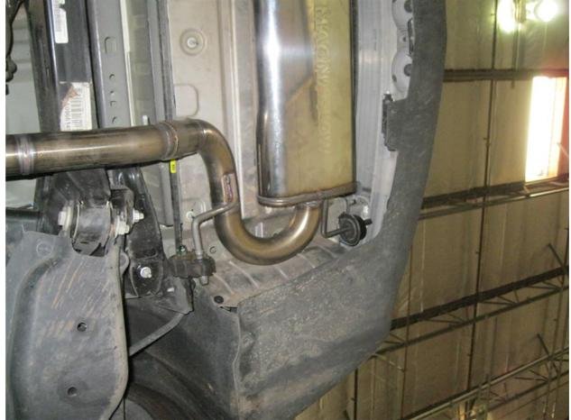
**Step 4.** Next, install the Muffler Assy to the Inlet Pipe Assembly using a supplied 2.25" clamp and fitting the hangers into the rubber insulators.
