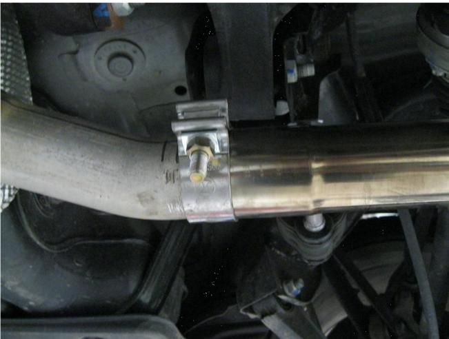
**Step 3.** Begin installation of your new MAGNAFLOW system by attaching the Inlet Pipe Assembly to the cut outlet behind the catalytic converter using the supplied 2.25" clamp (Keep all clamps loose until final adjustment) and insert hanger into rubber insulator.
