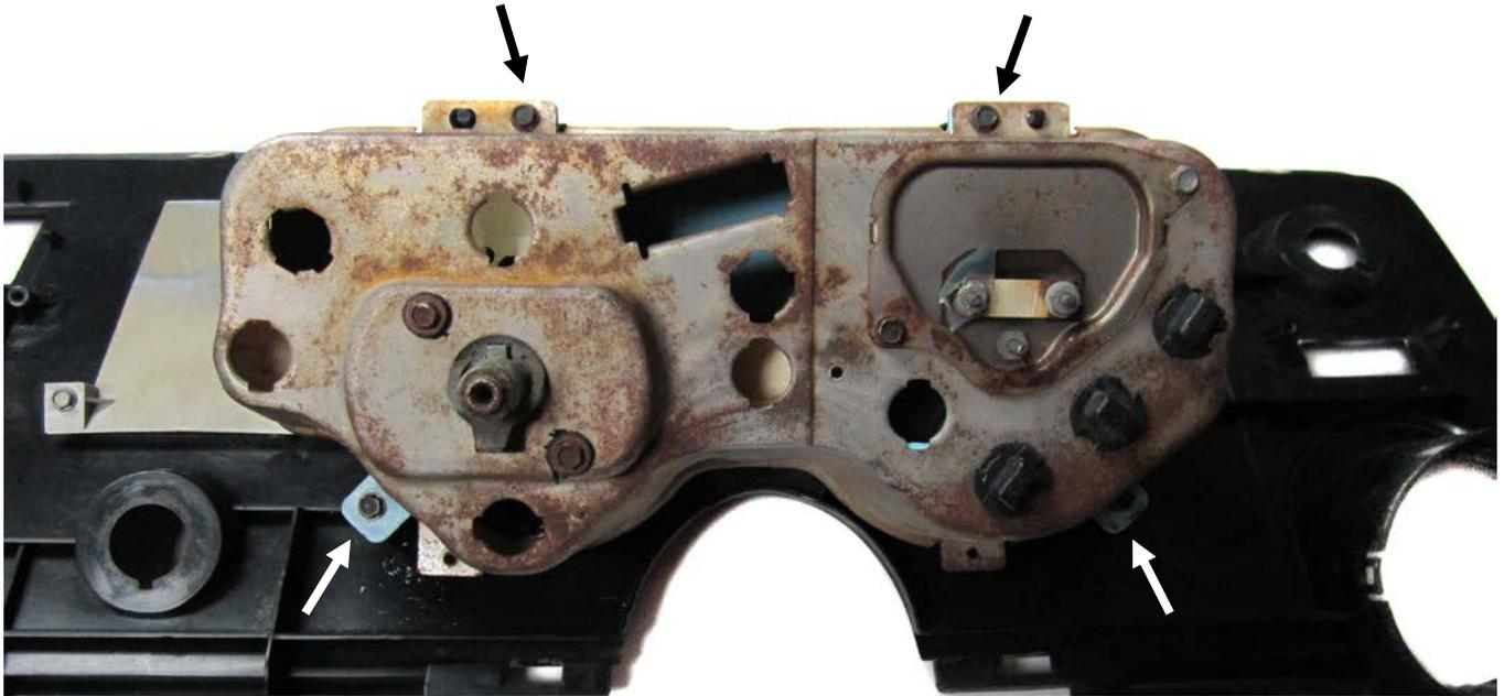
2. Install the Dakota Digital gauge to the factory dash. Using the four screws from step 1, secure the bezel paying special attention to make sure the gauges are properly centered in the bezel opening.
