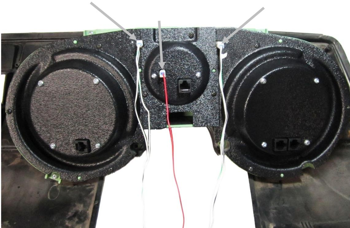
8. Make the CAT5 connections with one of the 36" cables to the back of the VHX system Speed and the other 36" cable to the back of the Clock. One end of the 24" CAT5 cable goes to the remaining jack on the Speed and the other end to the Tach. Both open ends of the 36" cables will be carefully routed to the control box mounting location during final assembly.
