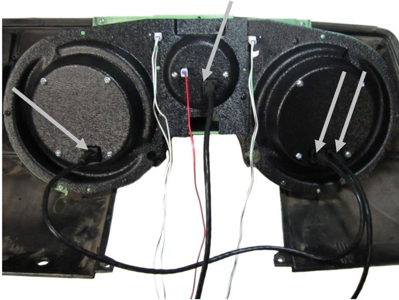
9. Reinstall the dash bezel and refer to the manuals 650314 and 650462 for wiring instructions to complete the VHX installation.
