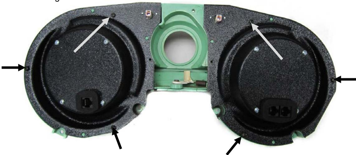
4. Install the remaining Clock instrument panel between the Speed and Tach, again using the supplied screws and washers.
