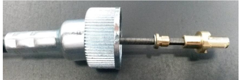
Cable inserted, brass tang in place
