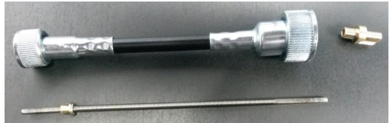
Inner cable removed
