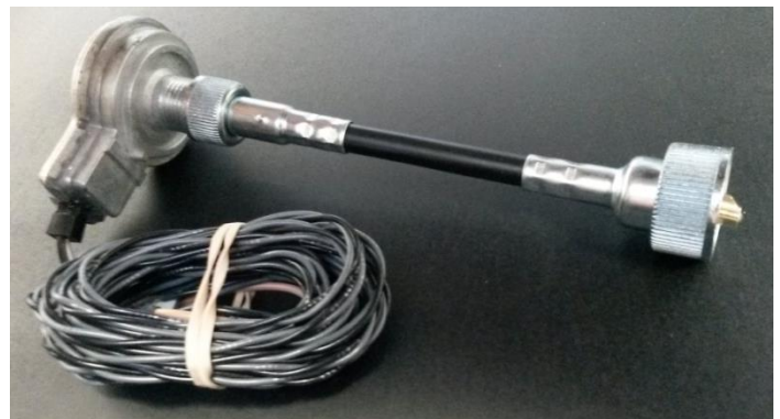
Sensor threaded on to cable assembly, ready for installation
