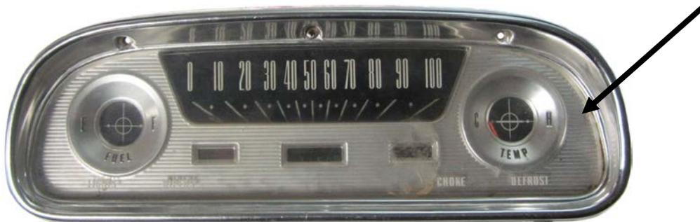
2. Remove the bezel by removing the two screws on the bottom and the one on top. Retain this hardware for reassembly. The bezel and housing along with their related mounting screws will be the only items reused.
