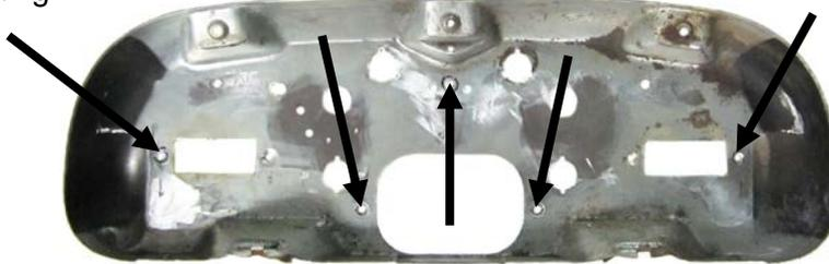
4. Carefully place the VHX system into the factory housing while aligning the studs coming out of the VHX system into the holes of the housing that were drilled in the previous step. Use the supplied nuts and lock washers to fasten the items together. Ensure the black ABS subpanel sits flush against the housing.
