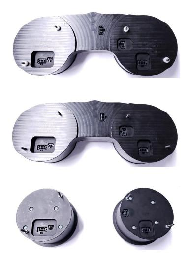
4. Insert Tach, Speed, Fuel & Volts gauges into the front of the bezel. Also insert the front half of the trim ring for the center Temp / Oil gauge.
