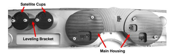
7. Connect the provided interconnect harness to the Speed, Temp / Oil and Tach gauges. Connect the satellite Fuel and Volts gauges to the rest of the system using the provided Y-harness.
