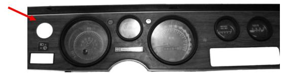
2. Remove the stock gauges and trim rings from the bezel. These items will not be reused and can be set aside.
