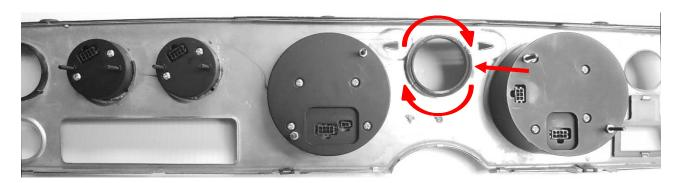
6. Slide the rear main housing over the speed and tach gauges and fasten into place using the provided thumb nuts. Then use the provided cups, leveling bracket and thumb nuts to secure the two satellite gauges in place.
