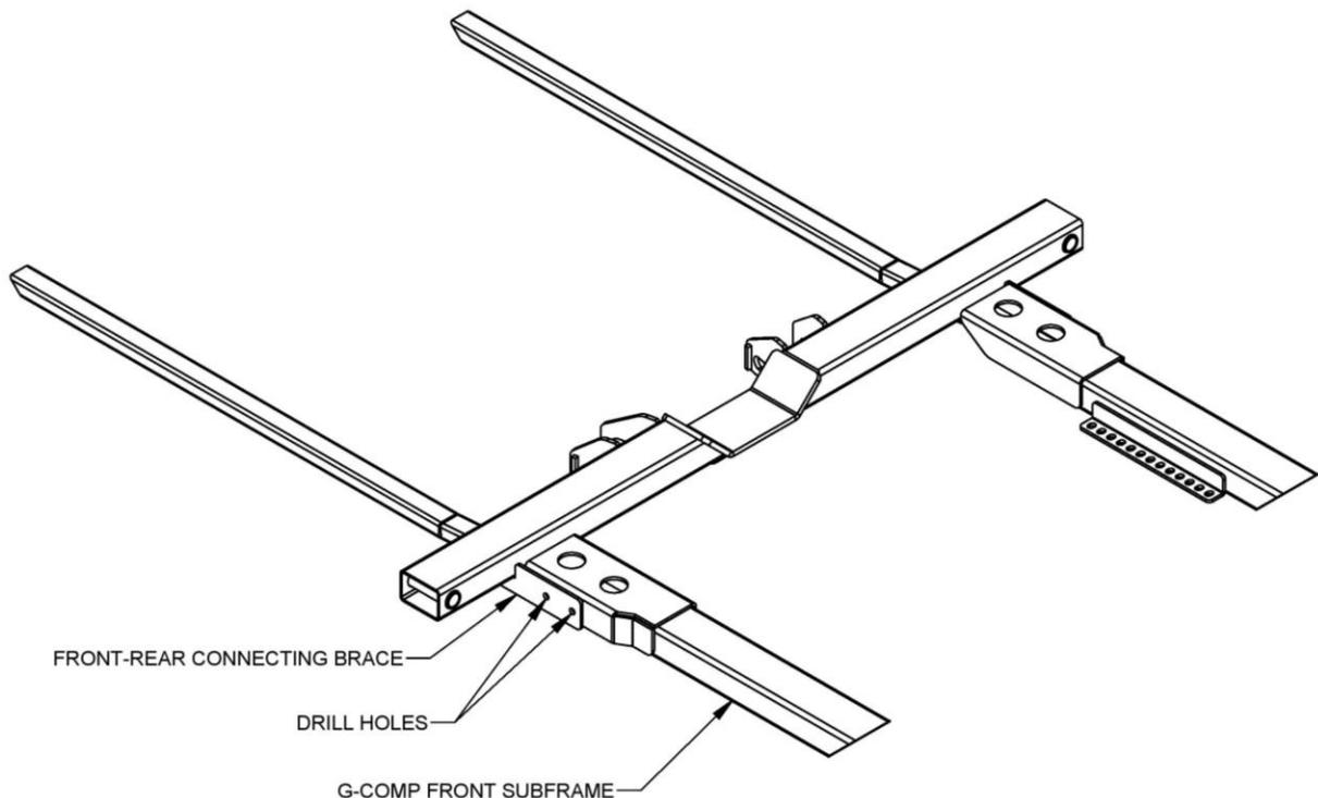
10. **Weld:** If there are no clearance issues, it is time to fully weld in the crossmembers. Start by removing the rear end, watts link, and truck arms from the car. Take note which link rod goes on which side. Fully weld the cross members and chassis braces to the car. **NOTE:** It is a good idea to only weld a small bead at a time, then move to a new area and allow the first area to cool completely before welding further in that area. This will greatly reduce the risk of warping.
