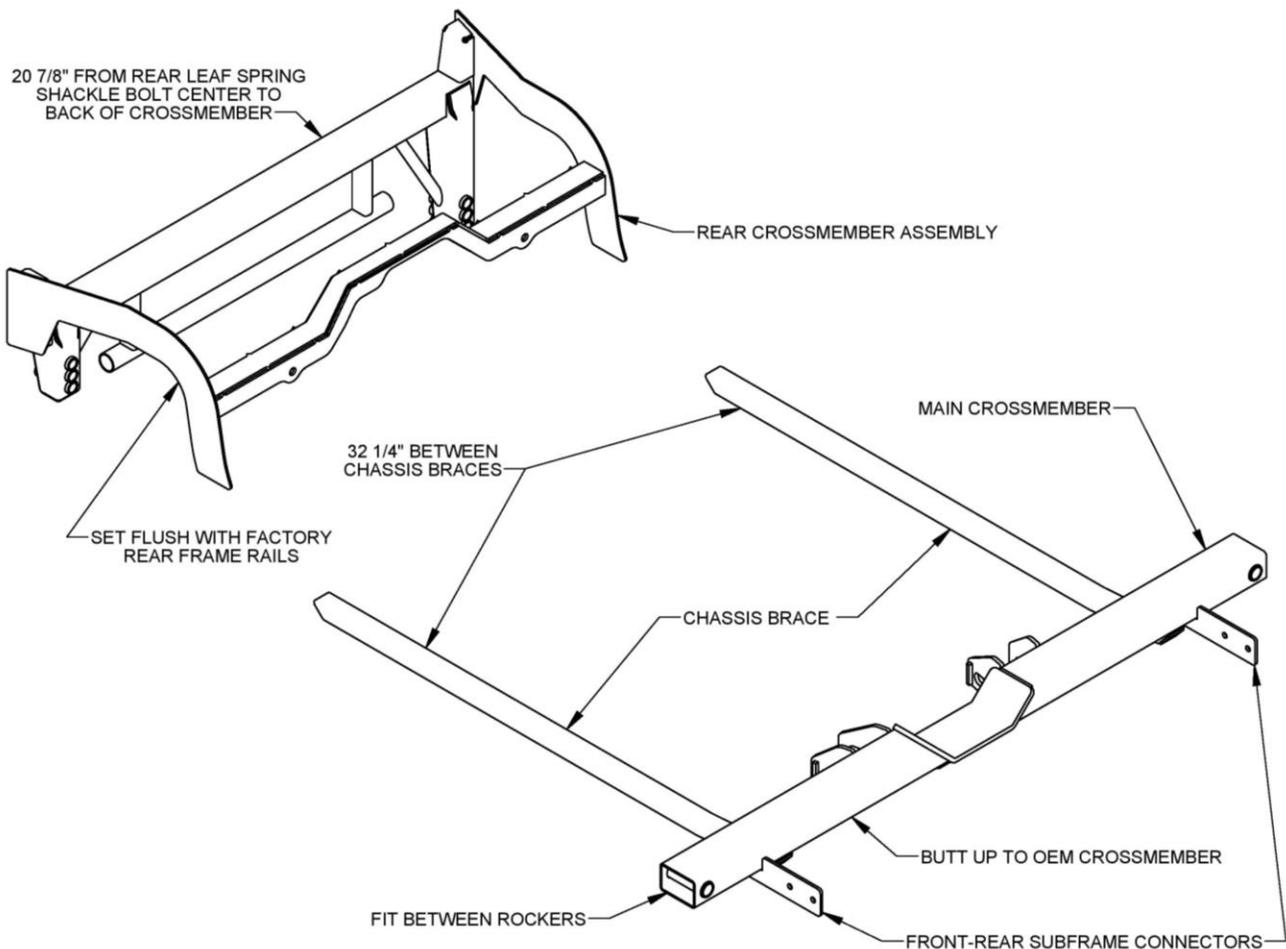
3. **Repeat** step two with the rear crossmember assembly. Depending on the car, minor trimming/fitting may be required. The rear crossmember assembly will sit between the factory rear frame rails and sit against the floor of the car. The rails should be flush with the outer plates of the assembly and the rear crossmember should be 20 7/8" from the factory rear leaf spring shackle bolts.
