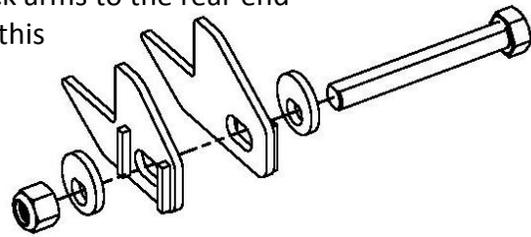
6. **Install the Watts Link Pivot:** Once the truck arms have been connected to the rear end housing, it's time to mock up the watts link. Start by installing the center pivot to the rear end housing. Use the supplied  $3/4$ -16 x 3" grade 5 bolt and washer to attach the pivot to the housing as shown. For initial mock up, use the second hole from the top on the rear end housing.
