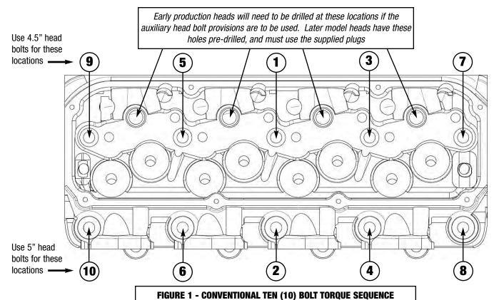
Bolts should be tightened to 100-110 ft/lbs in three intermediate steps. Applications using the eight (8) auxiliary bolt provisions should consult their engine block manufacturers instructions for the correct torque sequence.
