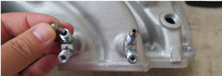
2. Install the passenger side Nitrous Assembly (Blue Assembly) onto the E2 nozzles. Nozzles are marked "N" for nitrous and "F" for fuel. Hand tighten all fittings, then use a 7/16" wrench to snug down the fittings.
