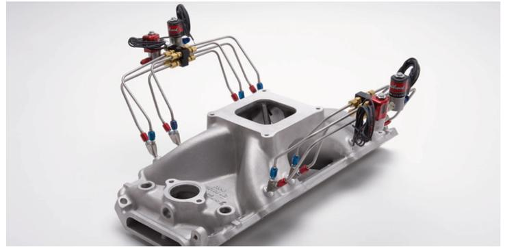
4. Remove any sensors on the factory manifold and install them onto the Edelbrock manifold. The 1/2" NPT fittings on the manifold must be plugged if not being used.
