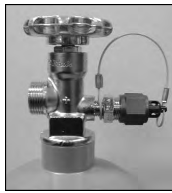
Installed on this valve is the Racer Safety Blow Off Adapter and Diffuser Cap. Whenever the bottle is not installed in the vehicle, be sure the Diffuser Cap is installed on the PRD. Also, be sure never to overtighten the Diffuser Cap or Blow Down Tube on the PRD.
