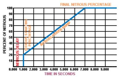
Nitrous Delay Timer = 1.000 seconds Nitrous Starting Percentage = 20% Final Nitrous Percentage = 100% Nitrous Power Ramp Time = 6.000 seconds
