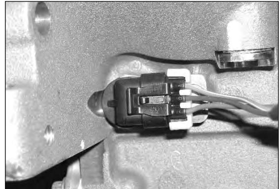
**Figure 5 - Crankshaft Position Sensor**
