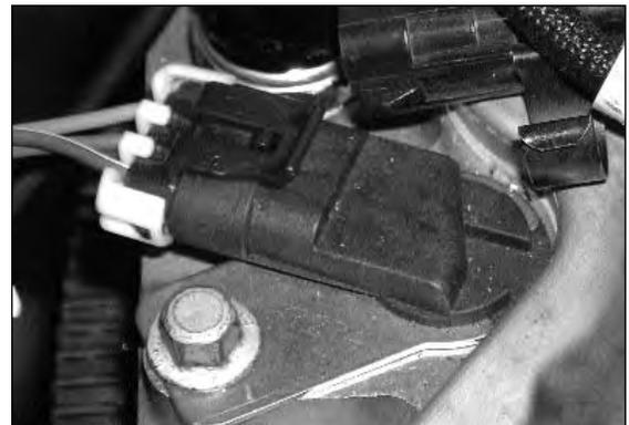
**Figure 6 - Camshaft Position Sensor**
